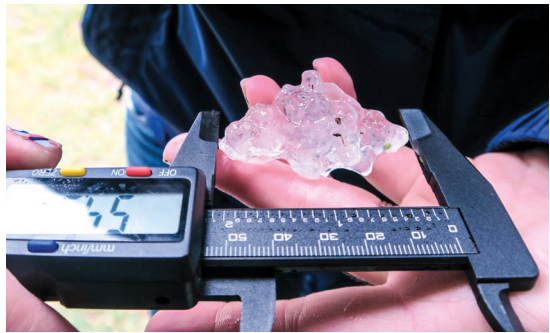
A researcher from the Tampa-based Institute for Business and Home Safety (IBHS) conducts an analysis of a freshly fallen hailstone before it begins to melt and its properties change.
